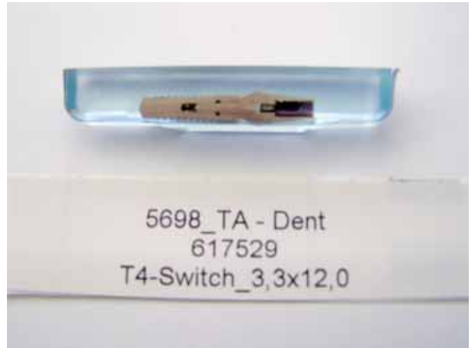
Figure no. 2: embeded assembly
