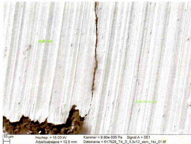
Figure no. 9: SE image - detail - head of the fixation screw - see figure no. 8; magnification: 1000x
