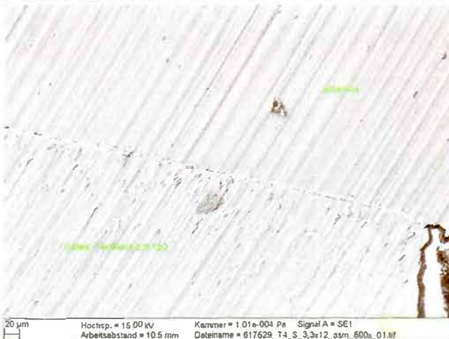
Figure no. 7: SE image - detail implant / abutment gap - see figure no. 6; magnification: 500x
